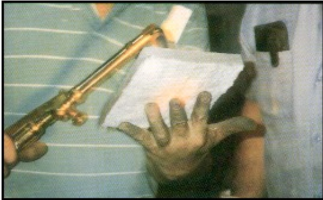
Fiber square coated with ITC-100 HT being torch tested
