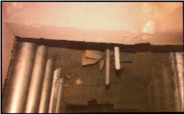
Radian heat tubes, fan, thermocouples and interior coated with ITC products
