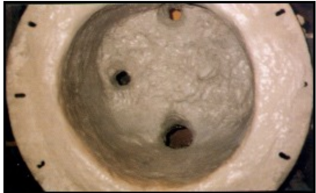
Tundish repaired with ITC-100, 148 and 296A
